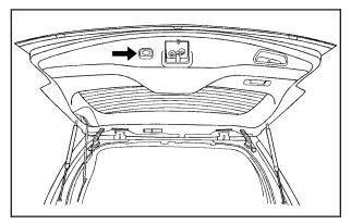
The liftgate can also be power closed by pressing the power liftgate button next to the liftgate latch. Press the button a second time during liftgate operation to reverse that operation. The power liftgate may be temporarily disabled under extreme temperatures or low battery condition. If this occurs, the liftgate can still be operated manually.
